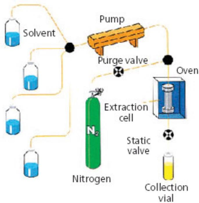
Schematic of a pressurized fluid extractor. (Accelerated Solvent Extractor, Dionex, Sunnyvale, California.)
